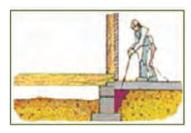
**Slab Foundations:** We insert the product under the foundation by drilling every 12 inches to encircle the entire building in areas where you have tile, brick or other decorative material. We are able to use our **Kil Foam** process in both cases. This system provides a continuous
